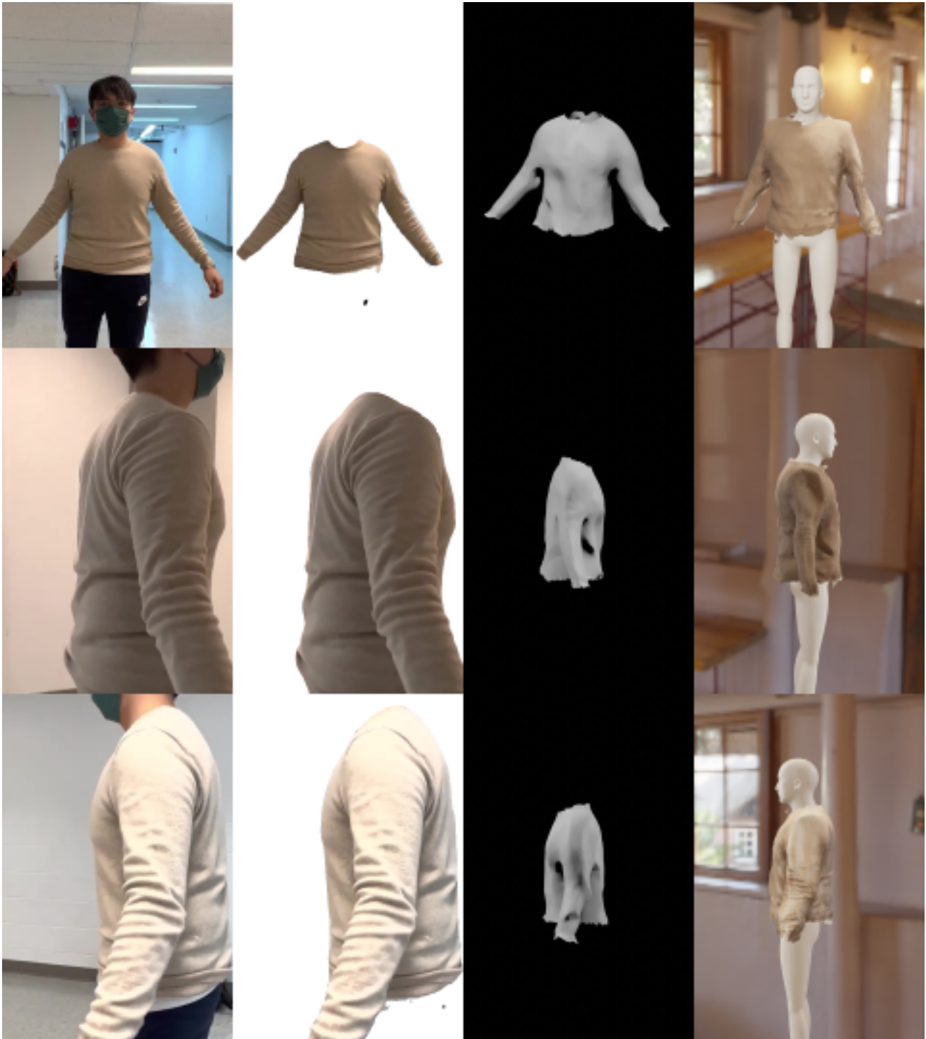
Figure 5: Sample output of each stage across 3 frames. From left to right - input sequence, extracted garment, reconstructed mesh and fitted garment on mannequin in Blender.
